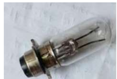
6V, 15Watt Halogen Lamp for Carl Zeiss Microscope
