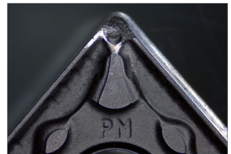
Indexable insert, shows tool wear. Reflected light, ringlight, zoom 0.8x
